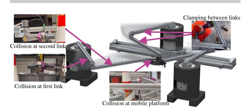
$\bullet$  Collision at the structure and clamping between links at velocities of  $0.4-0.9\,\mathrm{m/s}$
