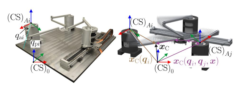
Kinetostatic projection of an arbitrary contact location to the platform and actuators
